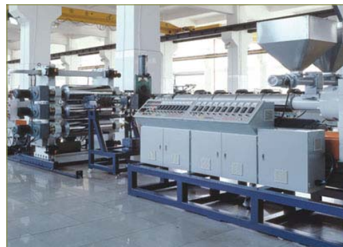
Polyethylene sheet extrusion
