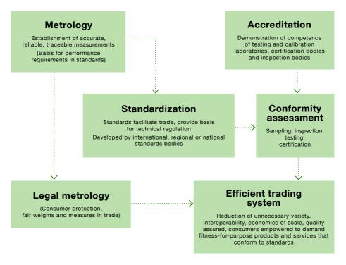
Figure 1 - How metrology, standardization and conformity assessment are interlinked
