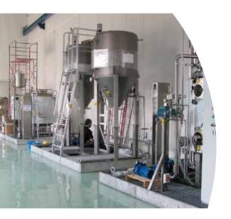
"We are the first country in the region to establish a PCB treatment facility, enabling the decontamination and reuse of PCBs-laced transformer oils."
