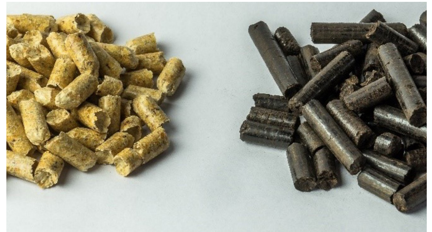
White pellets from debarked wood and black pellets from torrefied wood. (Source: Futerra Fuels)
