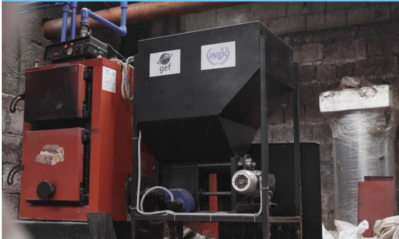
Combustion system for dried olive pomace in an olive factory. (Source: BEA)
