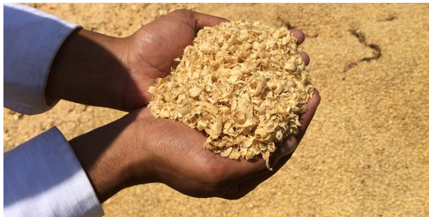
Gelan distillery boiler is able to burn low-grade biomass such as sawdust and coffee husk. (Source: Project Gaia Inc.)
