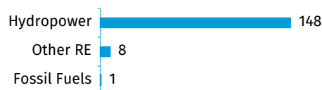
Figure 2. Annual Electricity Generation by Source in the Central African Republic in 2019 (GWh)
